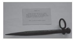
This cast-iron picket pin was used during the war to keep horses from wandering when no fenced area was available. The pin, which is approximately a foot in length, was driven into the ground, then the horse was tethered to the loop on the pin. This picket pin was reportedly used by Confederate troops at an encampment in Orange County.
